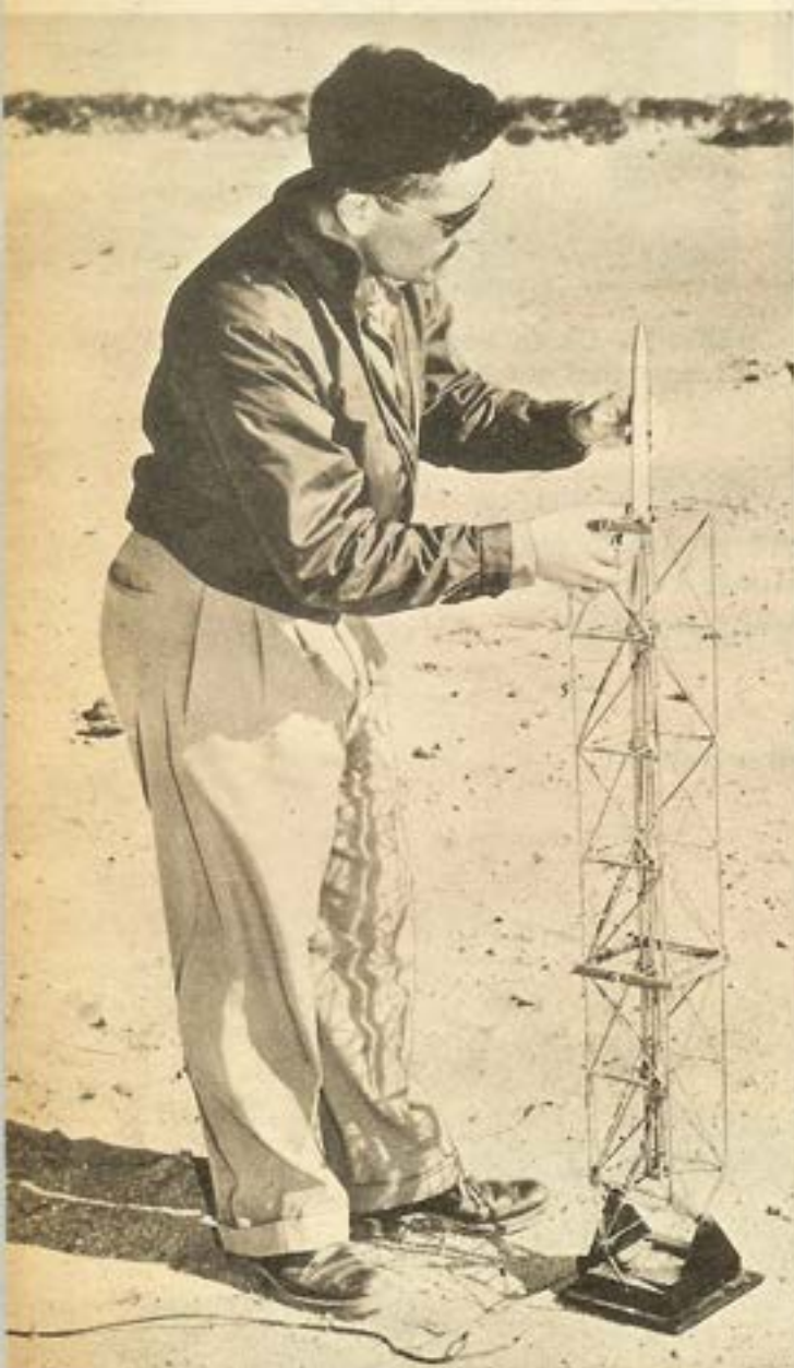
AEROBEE scale model being loaded in tower by author Stine is powered by basic Rock-A-Chute motor.
