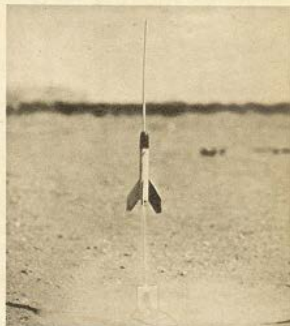
MISSILE AWAY! Total absence of flame is indication of highly efficient rocket motor.
